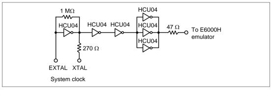
Figure 8 Clock Oscillator
